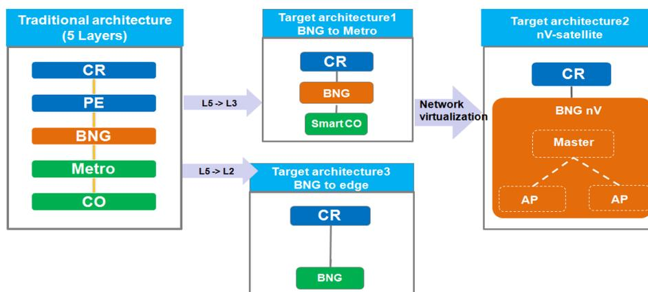
**Target architecture 1: BNG to metro (network delayed from five to three layers)**
