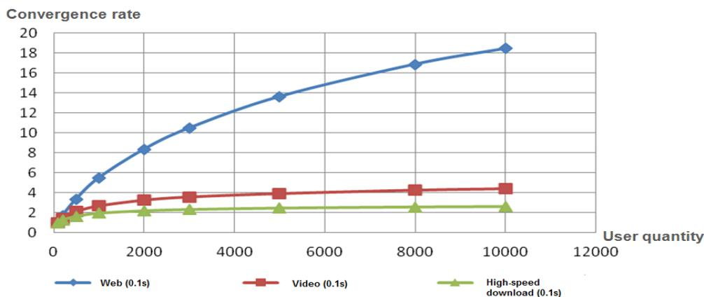
Faced by the traffic surge and change in the convergence model, the legacy network that has high aggregation and convergence rates present the following characteristics when bearing 4K video:
