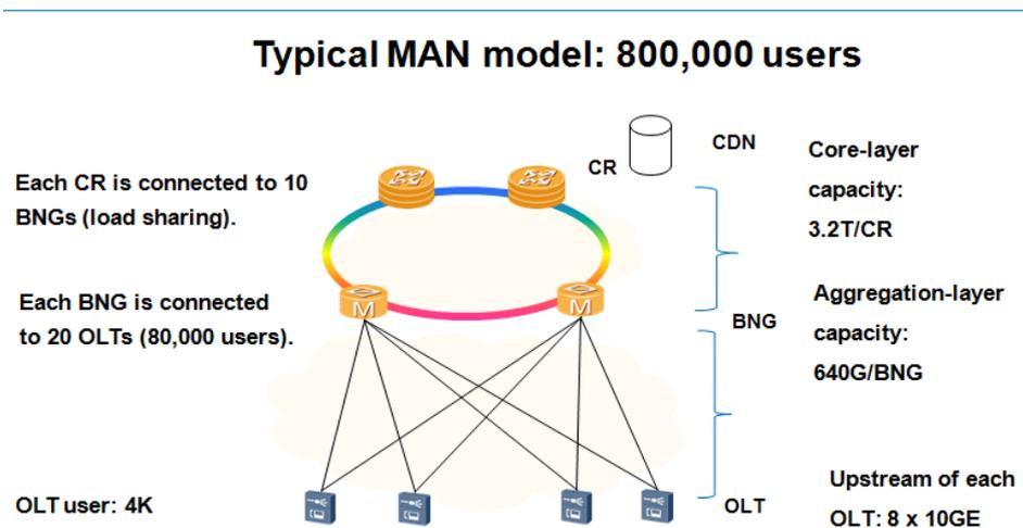
On a traditional network with direct fiber connections, each OLT uses four 10GE ports to connect to each BNG. Therefore, 80 pairs of fibers ( $20 \times 4$ ) are required between each BNG and OLT, and a total of 800 ( $10 \times 80$ ) pairs of fibers are required.
