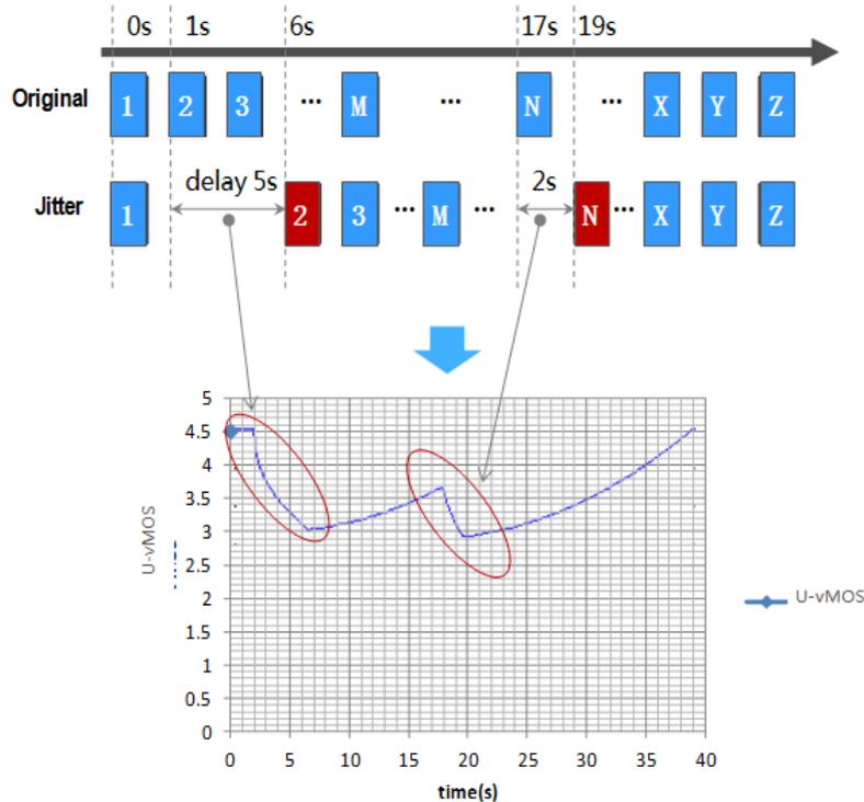
sView is determined by the following factors: Duration (average time required for a video stall), Interval (average time between two video stalls), and Frequency (number of video stalls).
