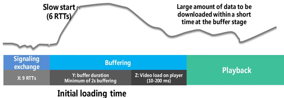
Considering that TCP slow start requires six RTTs and the download rate is typically low within this period, the entire download time requires at least seven RTTs. Specifically, the initial buffering time should be  $9 \text{ RTTs} + (6 + 1) \text{ RTTs} + 200 \text{ ms} \leq 1000 \text{ ms}$ , with each  $\text{RTT} \leq 50 \text{ ms}$ .
