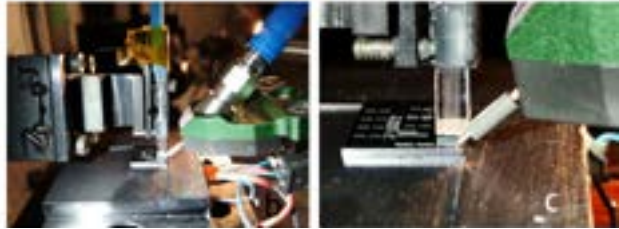
Figure 13 Testing setup. (a) Equipment diagram; (b) RF probe, fiber ribbon, and chip on the testing station; (c) Close-up view of the RF probe, fiber ribbon, and MRM die
