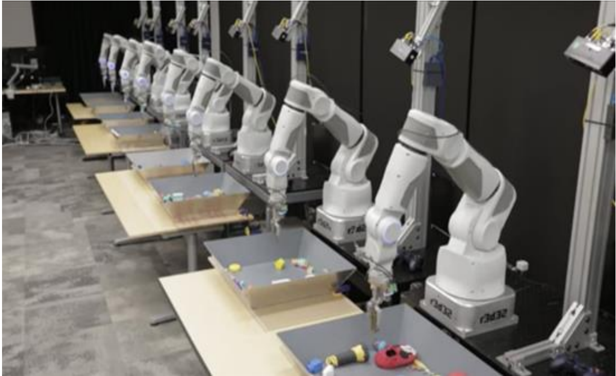
Figure 1: Large scale data collection with an array of robots (14 robots are sharing experiences of machine learning for grasping ) [Source: https://research.googleblog.com/2016/03/deep-learning-for-robots-learning-from.html ]
