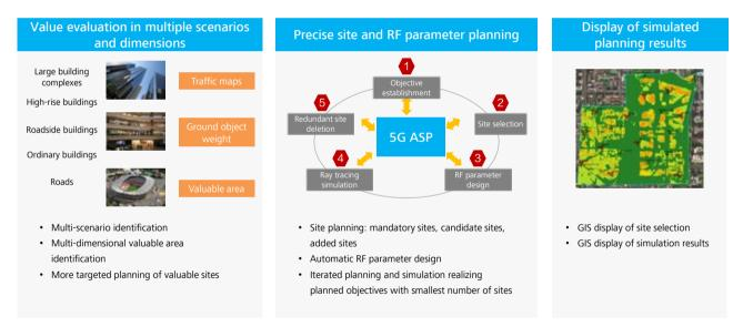
Figure 2-10 ASP functions for precise site planning
