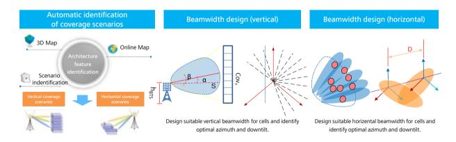
Figure 2-9 ACP functions for precise RF parameter planning
