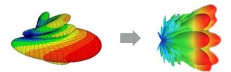
Figure 2-8 Traditional antenna pattern & Massive MIMO
