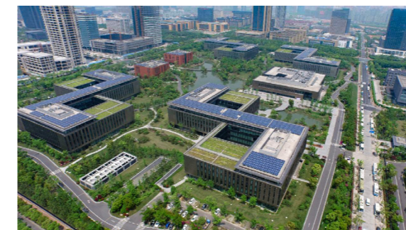
Smart PV plant at Huawei's Hangzhou Research Center Capacity: 1.8 MW Connected to the local grid in March 2015
