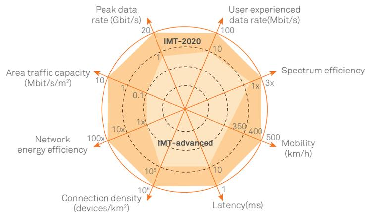
Figure 1: IMT-2020 usage scenarios and key capabilities
