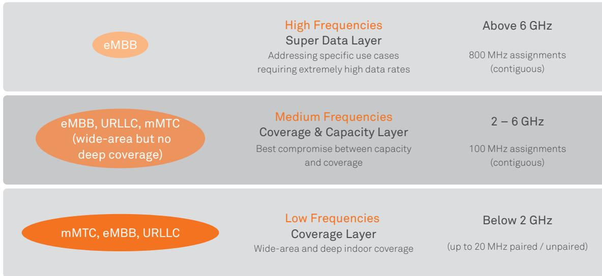
Figure 2: Multi-layer frequencies approach for 5G usage scenarios
