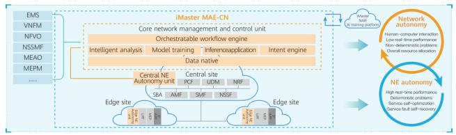
Figure 2-1 iMaster MAE-CN overall framework
