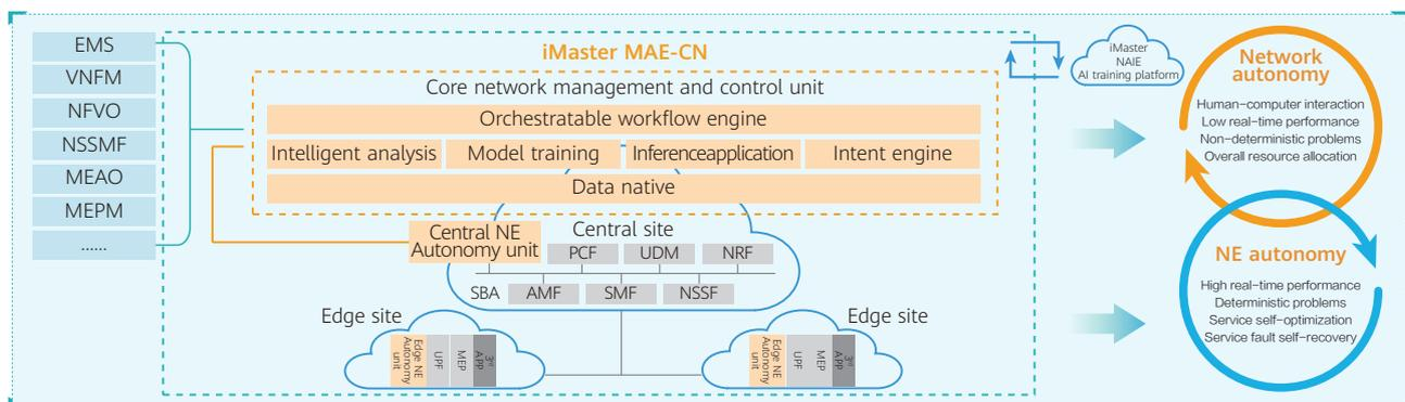
Figure 2-1 iMaster MAE-CN overall framework
