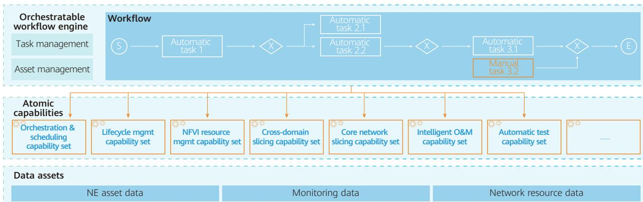
Figure 3-3 Atomic capability-based orchestration workflow
