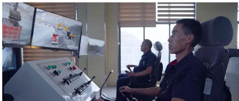
China Molybdenum workers remotely operating an excavator over a 5G network
