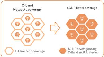
Figure 7: LTE/NR uplink spectrum sharing to extend 5G coverage at higher frequencies (e.g. C-band), accelerate deployment and reduce cost
