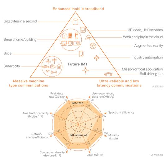
Figure 1: IMT-2020 usage scenarios and key capabilities Source: ITU-R
