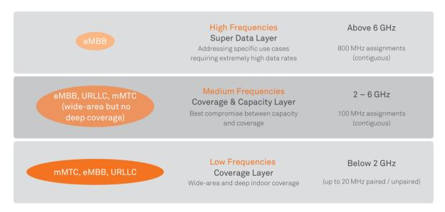
Figure 2: Multi-layer frequencies approach for 5G usage scenarios Source: Huawei
