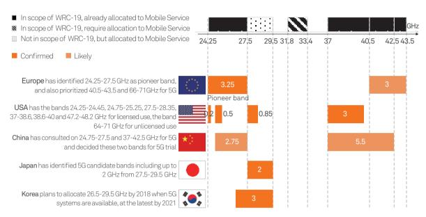
Figure 5: Frequency bands for early deployment of 5G millimetre wave systems Source: Hugwei
