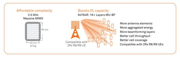
Figure 8: Massive MIMO affordable complexity Source: Huawei
