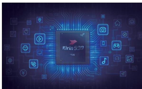
The Kirin 990 5G is manufactured using the cutting-edge 7nm + EUV process, which provides the industry’s most competitive performance, energy efficiency, and transistor density. 10.3 billion transistors are packed into an area the size of a fingernail, making the Kirin 990 5G 2019’s most complex commercial 5G SoC, with the most transistors and the most complete functions.
