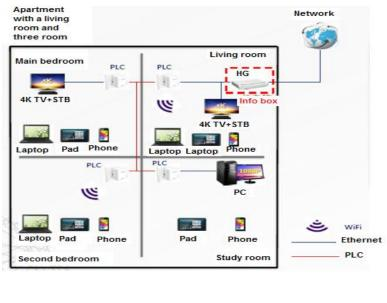
Figure 2-1 4K deployment for home networks in two typical apartment layouts
