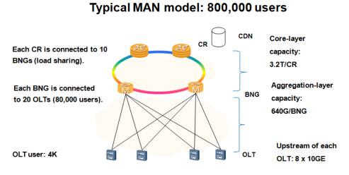
On a traditional network with direct fiber connections, each OLT uses four 10GE ports to connect to each BNG. Therefore, 80 pairs of fibers (20\*4) are required between each BNG and OLT, and a total of 800 (10\*80) pairs of fibers are required.
