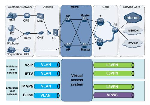
Figure 2-7 Typical application of virtual access
