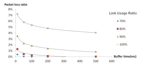
Figure 2-4 Relationship between the packet loss rate and link utilization
