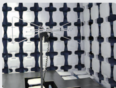
Laboratory for testing radio frequency signals emitted from mobile phones
