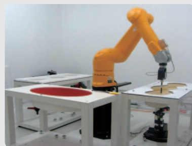
Laboratory for testing the specific absorption rate (SAR, an indicator of electromagnetic radiation) of devices
